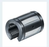
Super Linear Bushing A R0671..., open-type, with self-alignment feature Shaft diameter 12-50 mm With or without two integrated wiper seals, or with two integrated wiper seals and side seals (fully sealed)
