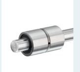
Torque-Resistant Linear Bushing R0724 2 with four ball guide grooves Shaft diameter 4–50 mm Hardened and ground outer sleeve, plastic ball retainer, keyway for torque transmission
