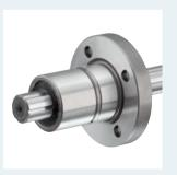
Torque-Resistant Linear Bushing R0725.., flanged, four ball guide grooves Shaft diameter 6–50 mm Hardened and ground outer sleeve, plastic ball retainer
