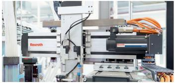
The flexible architecture of the EasyHandling system offers many ways to combine modules and implement applications.
